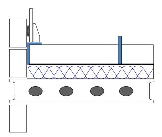
Expansion joints can be made using pre formed 8 or 10mm closed cell Polyethylene foam with a self-adhesive t-bar base known as a vertical control joint. Joints may be needed due to large areas, door thresholds or in between under floor heating circuits, this detail is particularly well suited to under floor heating as it eliminates cutting the screed.
